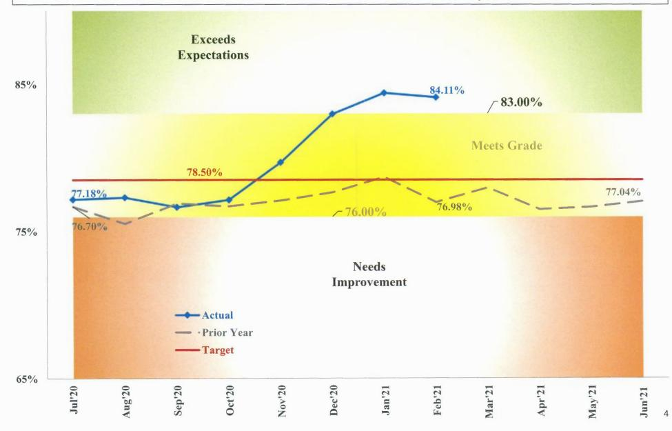
**Bus Mean Distance Between Failures** measured as the average actual vehicle miles (revenue + deadhead miles) between major mechanical failures reportable to NTD, except for those that occur at the end of the line.
