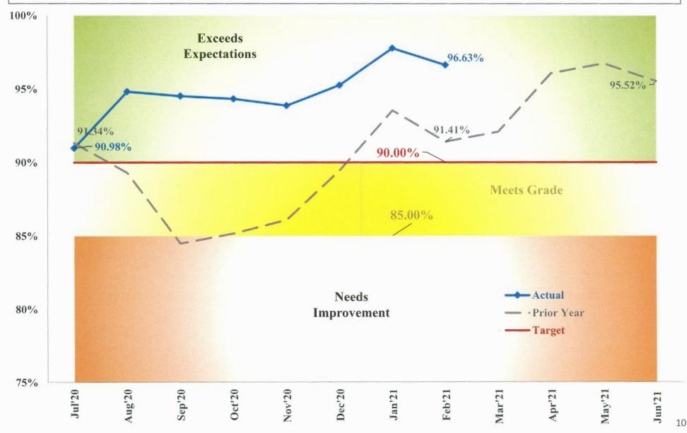
**Mobility Mean Distance Between Failures** measured as the average Mobility service miles between NTD reportable mechanical failures, i.e., those precluding a revenue vehicle from completing its revenue trip or starting its next scheduled revenue trip.
